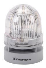
WERMA EvoSIGNAL Mini TwinLIGHT series LED audible-visual signal beacon, 95 dB at 1m, continuous/pulse tone(s), permanent or blinking (1 Hz ON for 470ms), clear/white, 62mm, 24 VAC/VDC, IP66. Requires mounting adapter.
