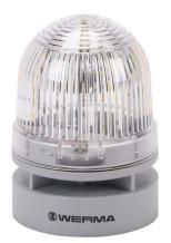
WERMA EvoSIGNAL Mini TwinLIGHT series LED audible-visual signal beacon, 95 dB at 1m, continuous/pulse tone(s), permanent or blinking (1 Hz ON for 410ms), clear/white, 62mm, 12 VAC/VDC, IP66. Requires mounting adapter.
