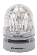
WERMA EvoSIGNAL Mini TwinLIGHT series LED audible-visual signal beacon, 95 dB at 1m, continuous/pulse tone(s), permanent or blinking (1 Hz ON for 410ms), clear/white, 62mm, 12 VAC/VDC, IP66. Requires mounting adapter.
