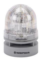
WERMA EvoSIGNAL Mini TwinLIGHT series LED audible-visual signal beacon, 95 dB at 1m, continuous/pulse tone(s), permanent or blinking (1 Hz ON for 420ms), clear/white, 62mm, 115-230 VAC, IP66. Requires mounting adapter.
