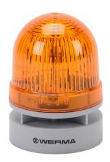
WERMA EvoSIGNAL Mini TwinFLASH series LED audible-visual signal beacon, 95 dB at 1m, continuous/pulse tone(s), double flash or EVS (Enhanced Visibility System) flashing (random flashing), yellow, 62mm, 24 VAC/VDC, IP66. Requires mounting adapter.
