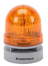
WERMA EvoSIGNAL Mini TwinFLASH series LED audible-visual signal beacon, 95 dB at 1m, continuous/pulse tone(s), double flash or EVS (Enhanced Visibility System) flashing (random flashing), yellow, 62mm, 12 VAC/VDC, IP66. Requires mounting adapter.
