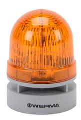
WERMA EvoSIGNAL Mini TwinLIGHT series LED audible-visual signal beacon, 95 dB at 1m, continuous/pulse tone(s), permanent or blinking (1 Hz ON for 470ms), yellow, 62mm, 24 VAC/VDC, IP66. Requires mounting adapter.
