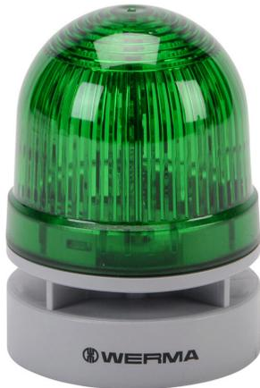
WERMA EvoSIGNAL Mini TwinFLASH series LED audible-visual signal beacon, 95 dB at 1m, continuous/pulse tone(s), double flash or EVS (Enhanced Visibility System) flashing (random flashing), green, 62mm, 115-230 VAC, IP66. Requires mounting adapter.
