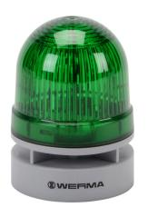
WERMA EvoSIGNAL Mini TwinLIGHT series LED audible-visual signal beacon, 95 dB at 1m, continuous/pulse tone(s), permanent or blinking (1 Hz ON for 470ms), green, 62mm, 24 VAC/VDC, IP66. Requires mounting adapter.
