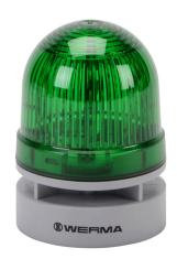
WERMA EvoSIGNAL Mini TwinLIGHT series LED audible-visual signal beacon, 95 dB at 1m, continuous/pulse tone(s), permanent or blinking (1 Hz ON for 410ms), green, 62mm, 12 VAC/VDC, IP66. Requires mounting adapter.
