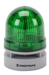
WERMA EvoSIGNAL Mini TwinLIGHT series LED audible-visual signal beacon, 95 dB at 1m, continuous/pulse tone(s), permanent or blinking (1 Hz ON for 420ms), green, 62mm, 115-230 VAC, IP66. Requires mounting adapter.
