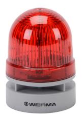
WERMA EvoSIGNAL Mini TwinFLASH series LED audible-visual signal beacon, 95 dB at 1m, continuous/pulse tone(s), double flash or EVS (Enhanced Visibility System) flashing (random flashing), red, 62mm, 12 VAC/VDC, IP66. Requires mounting adapter.
