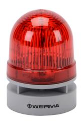
WERMA EvoSIGNAL Mini TwinLIGHT series LED audible-visual signal beacon, 95 dB at 1m, continuous/pulse tone(s), permanent or blinking (1 Hz ON for 470ms), red, 62mm, 24 VAC/VDC, IP66. Requires mounting adapter.
