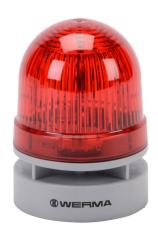
WERMA EvoSIGNAL Mini TwinLIGHT series LED audible-visual signal beacon, 95 dB at 1m, continuous/pulse tone(s), permanent or blinking (1 Hz ON for 410ms), red, 62mm, 12 VAC/VDC, IP66. Requires mounting adapter.
