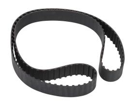
SureMotion timing belt, 3/8in L pitch, 1in wide, 120 tooth, 45in pitch length (circumference), neoprene, fiberglass reinforced.
