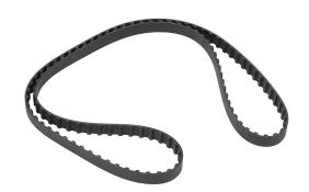
SureMotion timing belt, 3/8in L pitch, 1/2in wide, 120 tooth, 45in pitch length (circumference), neoprene, fiberglass reinforced.
