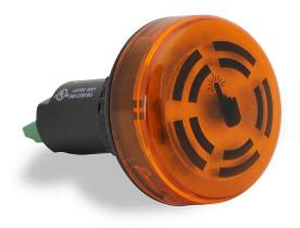
WERMA audible alarm buzzer, 80 dB at 1m, 2.8 kHz tone frequency, continuous tone(s), touch to acknowledge, 24 VDC, permanent LED indicator(s), yellow, 22mm, panel mount, polycarbonate housing, yellow, IP65.
