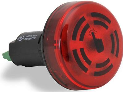
WERMA audible alarm buzzer, 80 dB at 1m, 2.8 kHz tone frequency, continuous tone(s), touch to acknowledge, 24 VDC, permanent LED indicator(s), red, 22mm, panel mount, polycarbonate housing, red, IP65.
