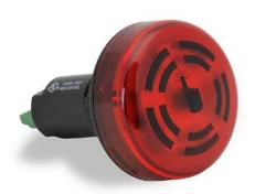
WERMA audible alarm buzzer, 80 dB at 1m, 2.8 kHz tone frequency, continuous tone(s), touch to acknowledge, 24 VDC, permanent LED indicator(s), red, 22mm, panel mount, polycarbonate housing, red, IP65.
