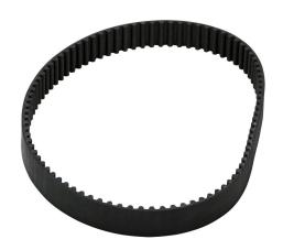
SureMotion timing belt, 5mm 5M pitch, 15mm wide, 90 tooth, 450mm pitch length (circumference), neoprene, fiberglass reinforced.
