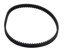
SureMotion timing belt, 5mm 5M pitch, 9mm wide, 90 tooth, 450mm pitch length (circumference), neoprene, fiberglass reinforced.
