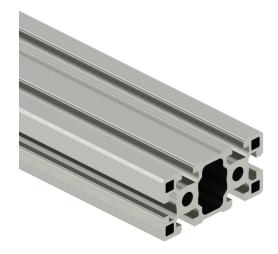
SureFrame 45 Series standard T-slotted rail, silver, 6063-T6 anodized aluminum alloy, cut to length, 45 x 90mm profile, slot size 10.
