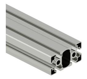
SureFrame 45 Series light T-slotted rail, silver, 6063-T6 anodized aluminum alloy, cut to length, 45 x 90mm profile, slot size 10.
