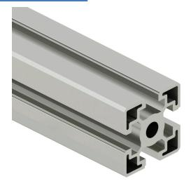
SureFrame 45 Series standard T-slotted rail, silver, 6063-T6 anodized aluminum alloy, cut to length, 45 x 45mm profile, slot size 10.
