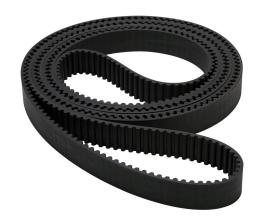
SureMotion timing belt, 8mm 8M pitch, 30mm wide, 550 tooth, 4400mm pitch length (circumference), neoprene, fiberglass reinforced.
