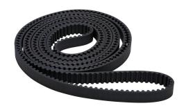
SureMotion timing belt, 8mm 8M pitch, 20mm wide, 550 tooth, 4400mm pitch length (circumference), neoprene, fiberglass reinforced.
