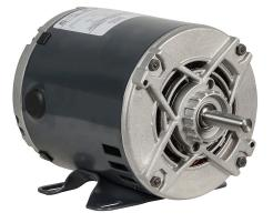
Marathon standard efficiency AC induction motor, general purpose, 1/4hp, 1-phase, 115 VAC, 1800rpm, ODP, NEMA 48 frame, rolled steel, rigid base mount.
