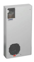
Seifert SlimLine air conditioner, 1770 BTU/H, R-134a, 115 VAC operating voltage, carbon steel housing, RAL 7035 light gray, filter-free, side mount. For use with NEMA 12 enclosures.
