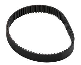
SureMotion timing belt, 5mm 5M pitch, 15mm wide, 85 tooth, 425mm pitch length (circumference), neoprene, fiberglass reinforced.
