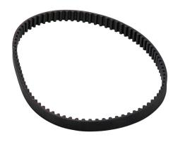
SureMotion timing belt, 5mm 5M pitch, 9mm wide, 85 tooth, 425mm pitch length (circumference), neoprene, fiberglass reinforced.
