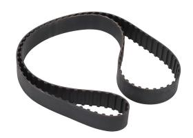
SureMotion timing belt, 3/8in L pitch, 1in wide, 112 tooth, 42in pitch length (circumference), neoprene, fiberglass reinforced.
