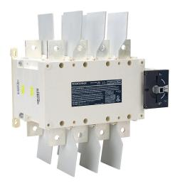
Socomec SIRCOVER series rotary manual transfer switch, 4-pole, 600 VAC, 400A, 65kA SCCR, panel mount, UL1008 rated, front operated, accepts 15 x 12mm size shaft.
