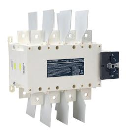
Socomec SIRCOVER series rotary manual transfer switch, 4-pole, 600 VAC, 260A, 65kA SCCR, panel mount, UL1008 rated, front operated, accepts 15 x 12mm size shaft.
