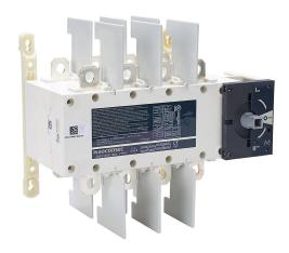
Socomec SIRCOVER series rotary manual transfer switch, 4-pole, 600 VAC, 100A, 100kA SCCR, panel mount, UL1008 rated, front operated, accepts 10 x 10mm size shaft.
