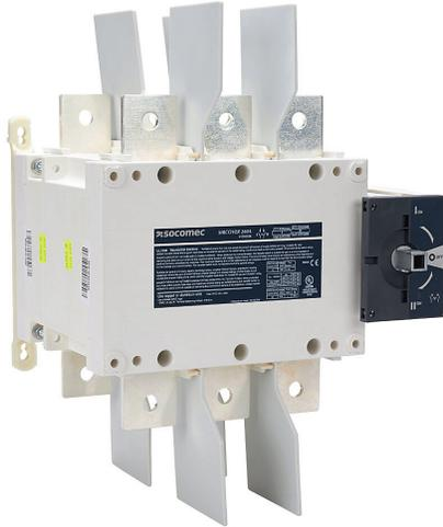
Socomec SIRCOVER series rotary manual transfer switch, 3-pole, 600 VAC, 260A, 65kA SCCR, panel mount, UL1008 rated, front operated, accepts 15 x 12mm size shaft.
