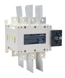
Socomec SIRCOVER series rotary manual transfer switch, 3-pole, 600 VAC, 260A, 65kA SCCR, panel mount, UL1008 rated, front operated, accepts 15 x 12mm size shaft.
