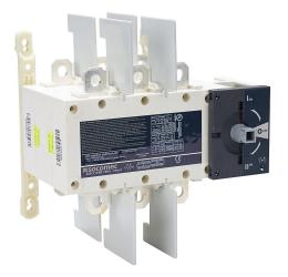
Socomec SIRCOVER series rotary manual transfer switch, 3-pole, 600 VAC, 100A, 100kA SCCR, panel mount, UL1008 rated, front operated, accepts 10 x 10mm size shaft.
