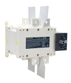
Socomec SIRCOVER series rotary manual transfer switch, 2-pole, 240 VAC, 260A, 65kA SCCR, panel mount, UL1008 rated, front operated, accepts 15 x 12mm size shaft.
