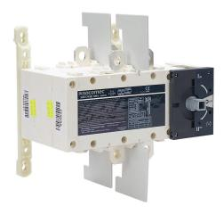
Socomec SIRCOVER series rotary manual transfer switch, 2-pole, 240 VAC, 100A, 100kA SCCR, panel mount, UL1008 rated, front operated, accepts 10 x 10mm size shaft.
