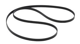
SureMotion timing belt, 0.08in MXL pitch, 1/4in wide, 400 tooth, 32in pitch length (circumference), polyurethane, polyester reinforced. Package of 3.
