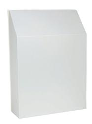
Seifert fan hood, fits 11.46 x 11.46in fan cutout, carbon steel, silicone gasket, NEMA 3R/4/12, IP56, for increasing the protection classification of side-mounted fans and grilles.
