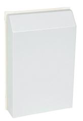
Seifert fan hood, fits 3.62 x 3.62in fan cutout, carbon steel, silicone gasket, NEMA 3R/4/12, IP56, for increasing the protection classification of side-mounted fans and grilles.
