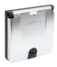
Murrelektronik Modlink panel interface frame, double frame, polyamide housing, black, single hinged, ABS plastic cover, metallic. For use with (2) Modlink series inserts.
