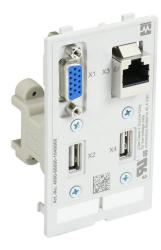
Murrelektronik Modlink panel interface insert, (1) RJ45 Cat5e female exterior/female interior, (1) 15-pin D-sub HD15 connector with female exterior/male interior and (2) USB A port with female exterior/female interior, single frame. For use with Modlink series frames.
