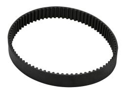
SureMotion timing belt, 5mm 5M pitch, 15mm wide, 80 tooth, 400mm pitch length (circumference), neoprene, fiberglass reinforced.
