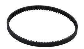
SureMotion timing belt, 5mm 5M pitch, 9mm wide, 80 tooth, 400mm pitch length (circumference), neoprene, fiberglass reinforced.
