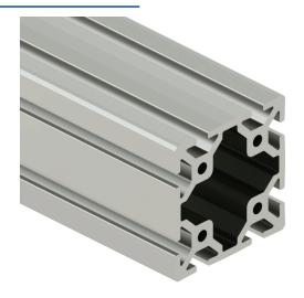
SureFrame 40 Series standard T-slotted rail, silver, 6063-T6 anodized aluminum alloy, cut to length, 80 x 80mm profile, slot size 8.
