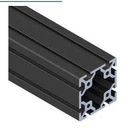
SureFrame 40 Series standard T-slotted rail, black, 6063-T6 anodized aluminum alloy, cut to length, 80 x 80mm profile, slot size 8.
