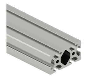
SureFrame 40 Series standard T-slotted rail, silver, 6063-T6 anodized aluminum alloy, cut to length, 40 x 80mm profile, slot size 8.
