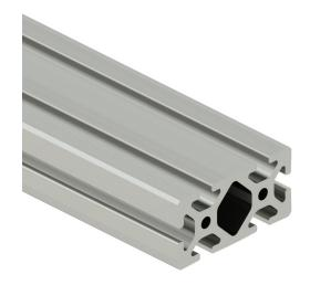
SureFrame 40 Series standard T-slotted rail, silver, 6063-T6 anodized aluminum alloy, cut to length,  $40 \times 80$ mm profile, slot size 8.
