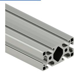
SureFrame 40 Series light T-slotted rail, silver, 6063-T6 anodized aluminum alloy, cut to length, 40 x 80mm profile, slot size 8.
