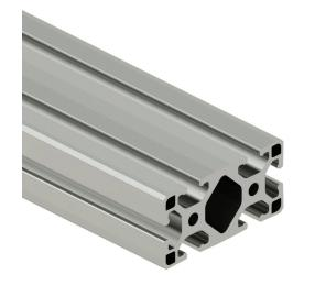
SureFrame 40 Series light T-slotted rail, silver, 6063-T6 anodized aluminum alloy, cut to length, 40 x 80mm profile, slot size 8.
