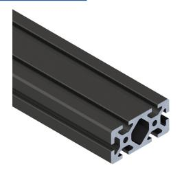
SureFrame 40 Series standard T-slotted rail, black, 6063-T6 anodized aluminum alloy, cut to length, 40 x 80mm profile, slot size 8.
