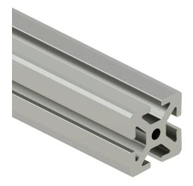
SureFrame 40 Series standard T-slotted rail, silver, 6063-T6 anodized aluminum alloy, cut to length, 40 x 40mm profile, slot size 8.
