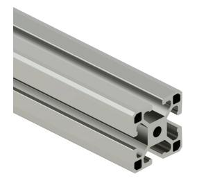
SureFrame 40 Series light T-slotted rail, silver, 6063-T6 anodized aluminum alloy, cut to length, 40 x 40mm profile, slot size 8.
